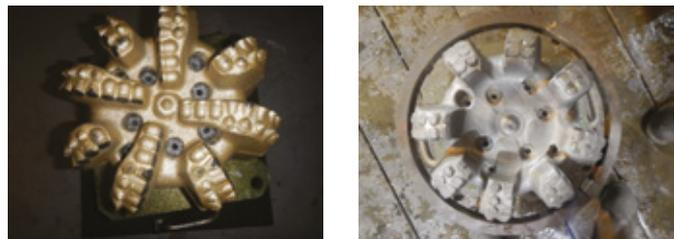
Figure 2. PDC bit shown before and after drill bit metamorphism. Bit on the right, note the center has completely broken off and the bit is under gauge. Metal left down hole can result in additional NPT for fishing operations, circulation to clear debris and damage to subsequent bits.
