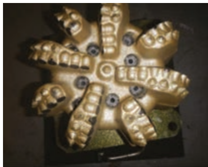
Fig. 1—GEOLOG's BitLife wear-monitoring service identifies the optimal time to pull a drilling bit on the basis of wear (left, a bit before wear; right, a bit pulled before excessive wear).
