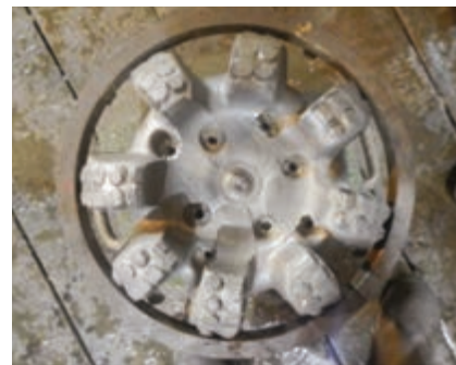
Fig. 1—GEOLOG's BitLife wear-monitoring service identifies the optimal time to pull a drilling bit on the basis of wear (left, a bit before wear; right, a bit pulled before excessive wear).
