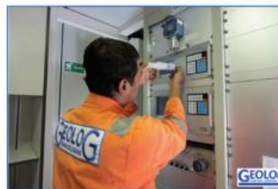
Fig. 5: Calibration of a Flame Ionization-type chromatograph for the measurement of hydrocarbons while drilling.
