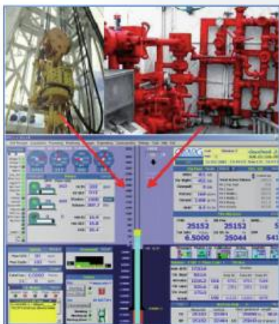
Fig. 2: Dozens of sensors connect the rig equipment to the Mud Logging data management system.
