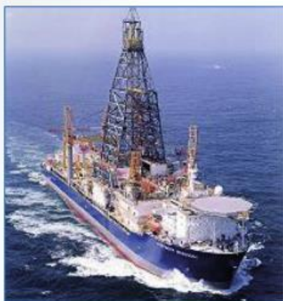
Fig. 3: Drillships are the most expensive drilling units and require advanced mud logging monitoring systems for their operational safety.
