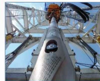
Fig. 2 - BHI's new LWD fluid sampler.
