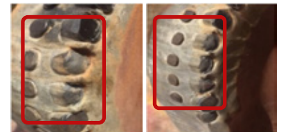
Under gauge bit with chipped teeth
