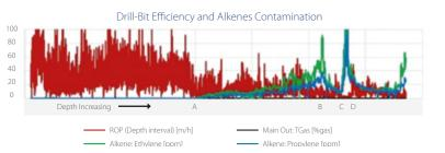
Figure 1. Drill Bit Efficiency plot highlighting ROP and detectable Alkenes. "Drill-Bit-Metamorphism" effect was observed starting at point A. Alkenes continue to increase until point B, indicating the ideal time to perform a bit trip. An additional increase in Alkenes occurs at point C, correlating to extremely low ROP before performing the bit trip. Point D marks the start of the new bit, which demonstrated extreme wear very quickly due to junk left in the hole.
