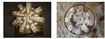
Figure 2. PDC bit shown before and after drill bit metamorphism. Bit on the right, note the center has completely broken off and the bit is under gauge. Metal left down hole can result in additional NPT for fishing operations, circulation to clear debris and damage to subsequent bits.
