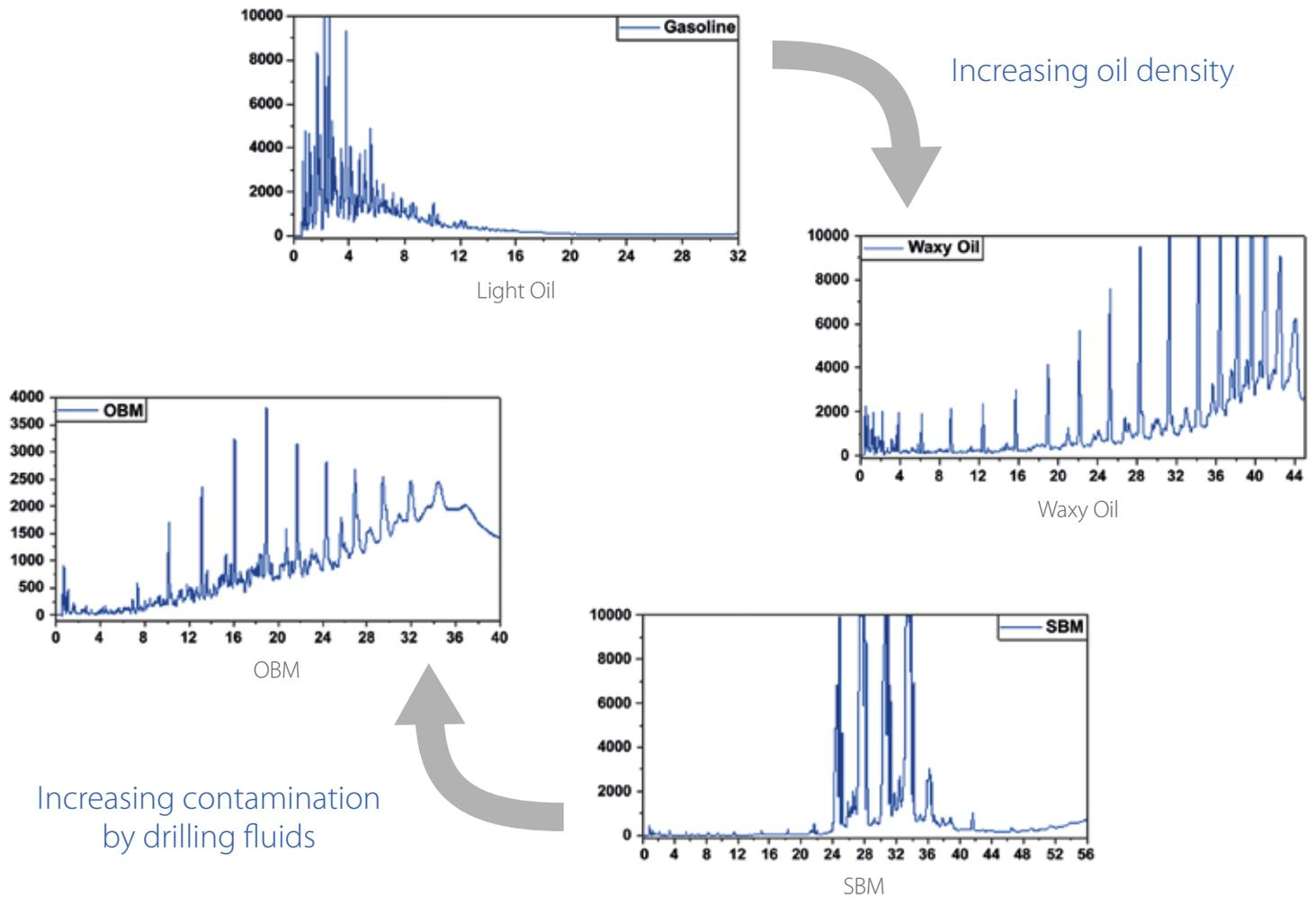
G9+ provides detailed analysis of cuttings for fluid characterization. As shown in the graphs above, the thermal desorption process can distinguish different fluid characteristics, helping the reservoir engineer better understand the reservoir fluid properties and at the same time identify the signatures of contaminating agents such as (synthetic) oil based muds.
