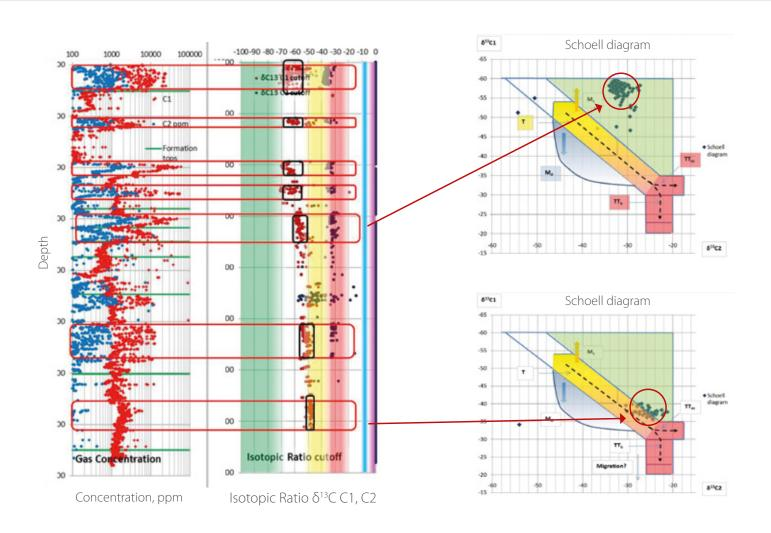
The log charts on the left identify different isotopic marking of gases detected at different well targets. The shallower ones indicate mixing with bacterial gas. Only the lowest interval (the main reservoir target) shows a clear thermogenic origin. On the right, the crossplots between C1 and C2 isotopic ratio show the extent of migration and alteration of the hydrocarbons. This is only possible on site with GEOLOG's Geolsotope service providing continuous well data and interpretation.
