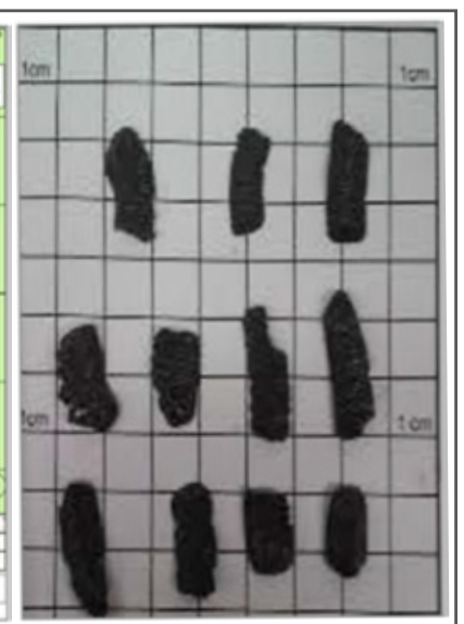
Figure 2. Shows the large blocky stress relief cuttings that were correctly identified during drilling
