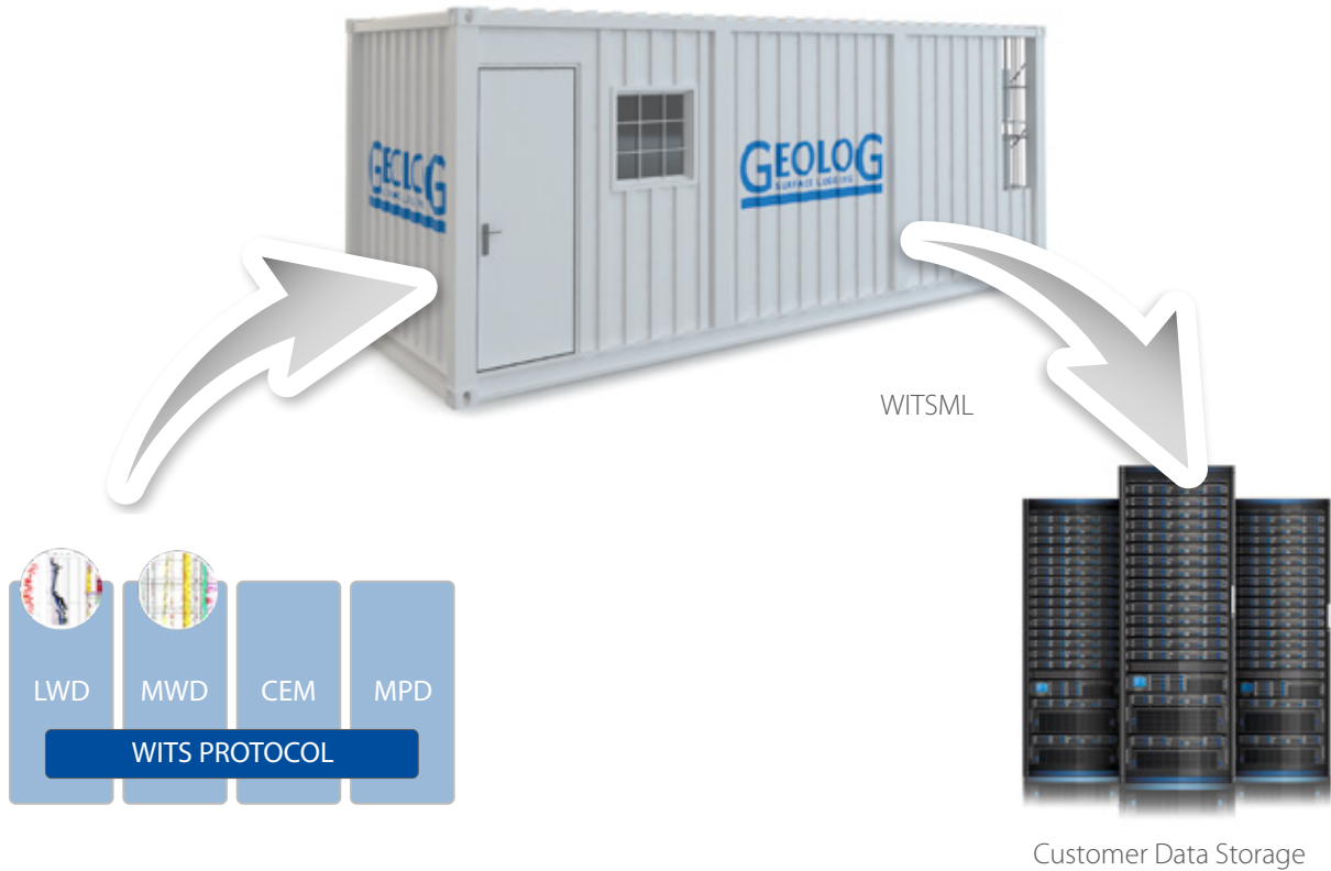
Figure 1. Schematic of the solution provided for the client. All WITS data collected through our unit on location, sent to our WITSML server with 24/7 support and then transmitted to client office for analysis.
